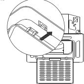
Step 4: Connect the 2 wires of the decoration panel to the mainboard of the unit.
