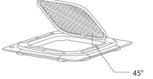
Step 2: Remove the installation covers at the four corners by sliding them outwards.
