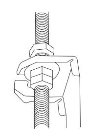
NOTE: The bottom of the unit should be 10-18mm(0.4-0.7")(Super-Slim models) or 24mm (0.9")(Compact models) higher than the ceiling board. Generally, L (indicated in the following figure) should be half the length of the suspension bolt or long enough to prevent the nuts from coming off.
