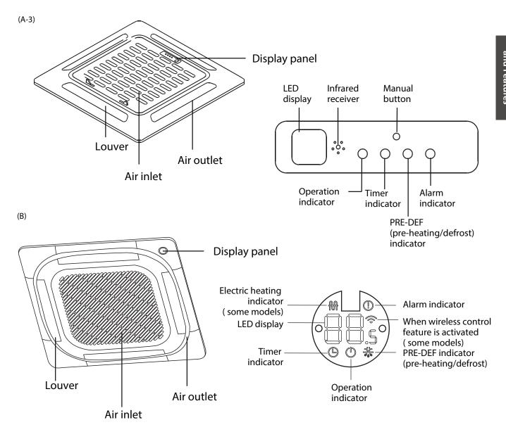
• MANUAL button: This button selects the mode in the following order: AUTO, FORCED COOL, OFF. FORCED COOL mode: In FORCED COOL mode, the Operation light flashes. The system will then turn to AUTO after it has cooled with a high wind speed for 30 minutes. The remote control will be disabled during this operation.
