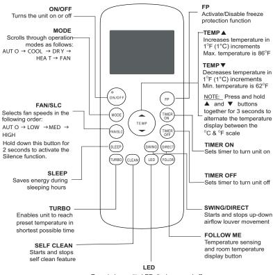
Turns indoor unit's LED display on and off. If you are sensitive to light when you go to sleep, you can press the LED button to turn off the LED display on the indoor unit. Press the button again to turn it back on
